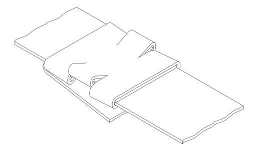
Sharp edged or misformed joints which do not appear as shown have to be taken away from the load immediately. The tensile strength of these joints is insufficient and they could cause serious injury. Having faulty joints proceed as follows:
